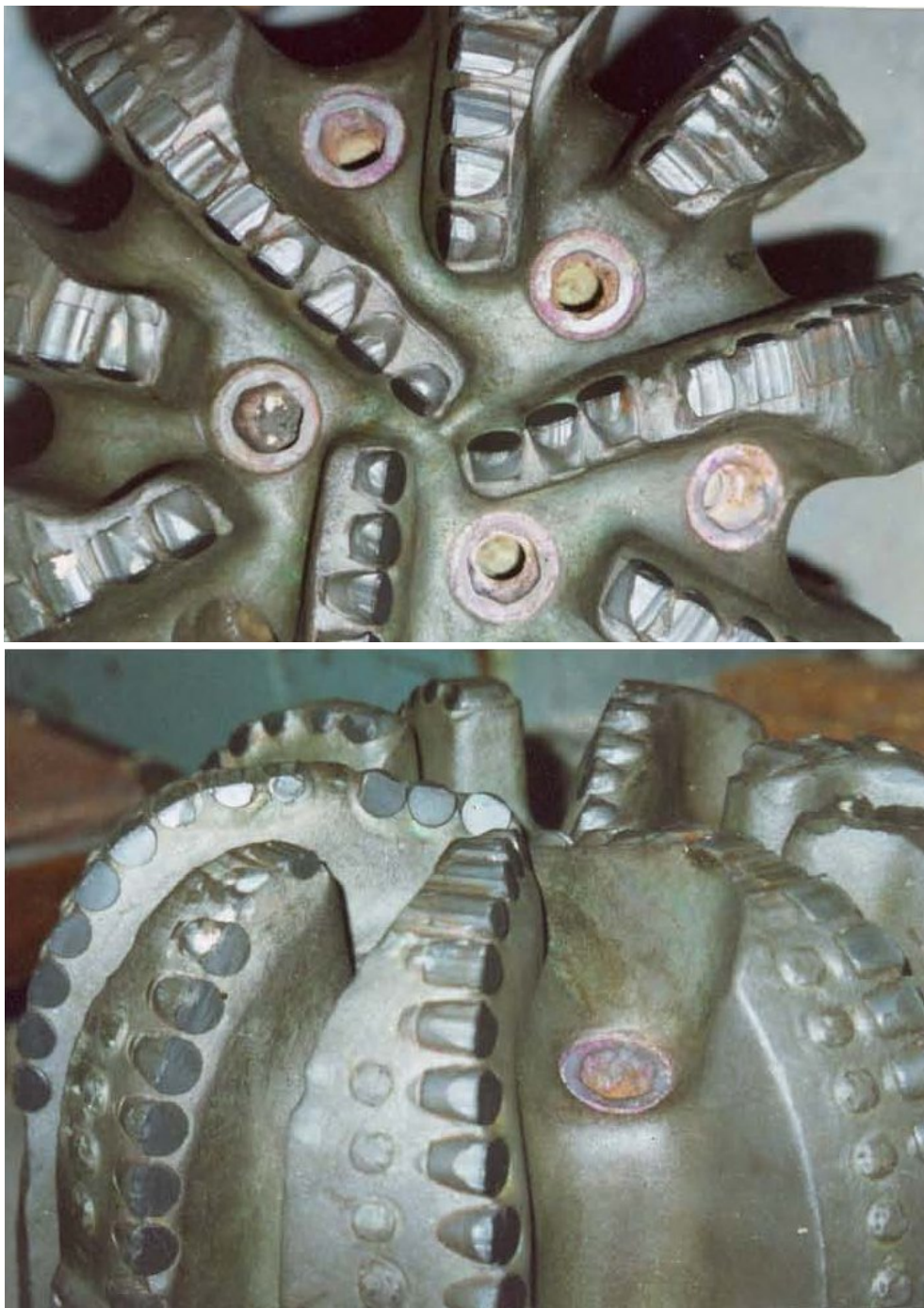
Figure 4. Photo of runned drill bit Read Hycalog 11 5/8 DS 66
